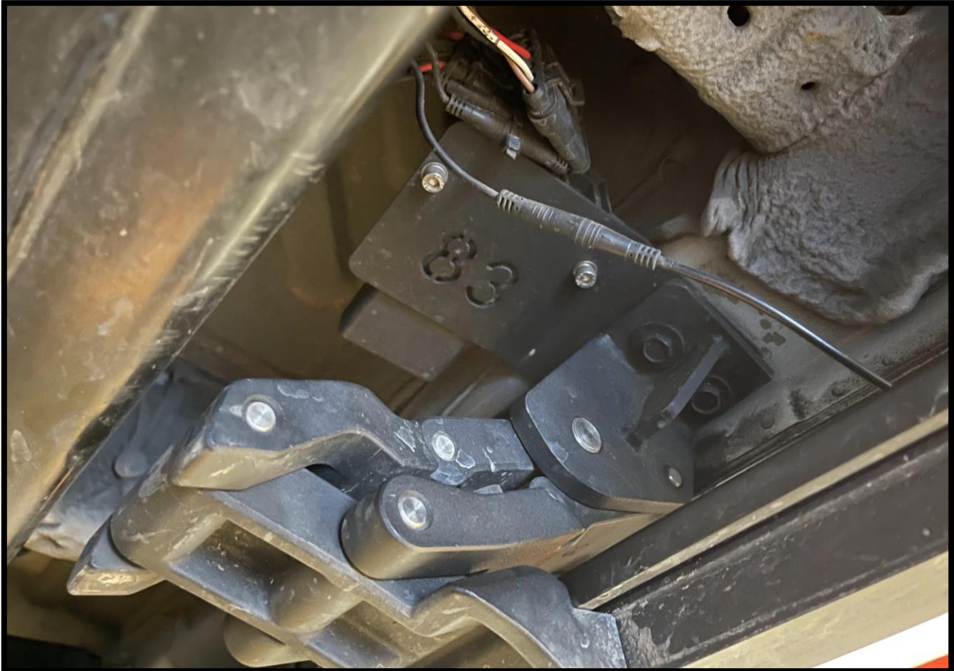
Step 6: Control module shown sandwiched onto center linkage.
